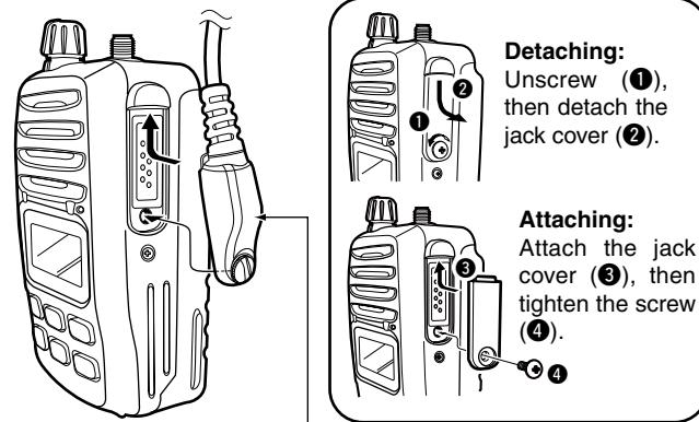
**CAUTION:** Attach the speaker-microphone's connector securely to prevent accidental dropping, or water intrusion in the connector.
