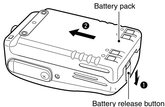
**CAUTION!** When pushing the battery release button, slide the battery pack slightly in the direction of the arrow (②) to ease release. This will prevent possible injuring to your fingers or nails
